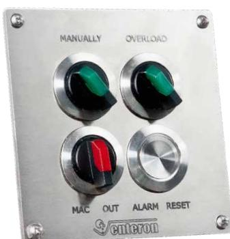
The remote control requires a panel cut-out of 65 mm x 65 mm or 80 mm hole circle; the base plate measures 95 mm x 95 mm and is attached to the corners with the supplied small wood screws.
